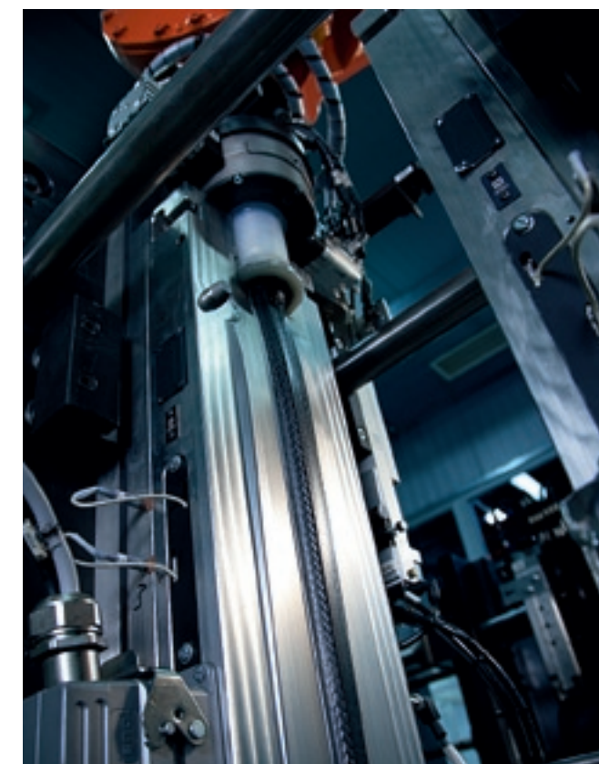
Resin is added to the frame tubes of the impec in these molds.
